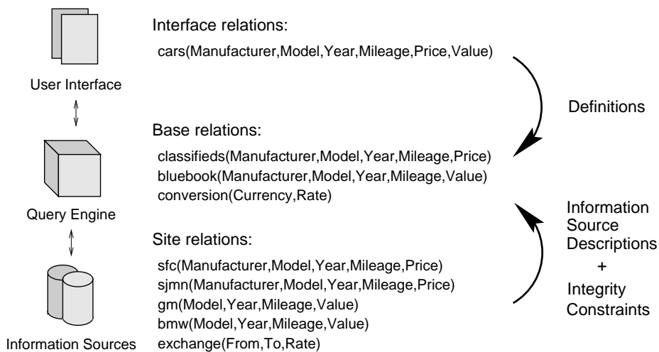
Figure 2: The information integration problem is abstracted as describing the relationships between three kinds of relations: Interface relations conceptualize the interaction with a user through a WWW based user interface. Site relations represent the data that is actually stored in the available information sources. Base relations are used as means to describe both interface and site relations and are crucial in the query planning process.
